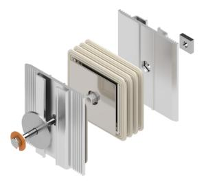
Note: Joint double-headed bolt torque value is 68±7 Nm
