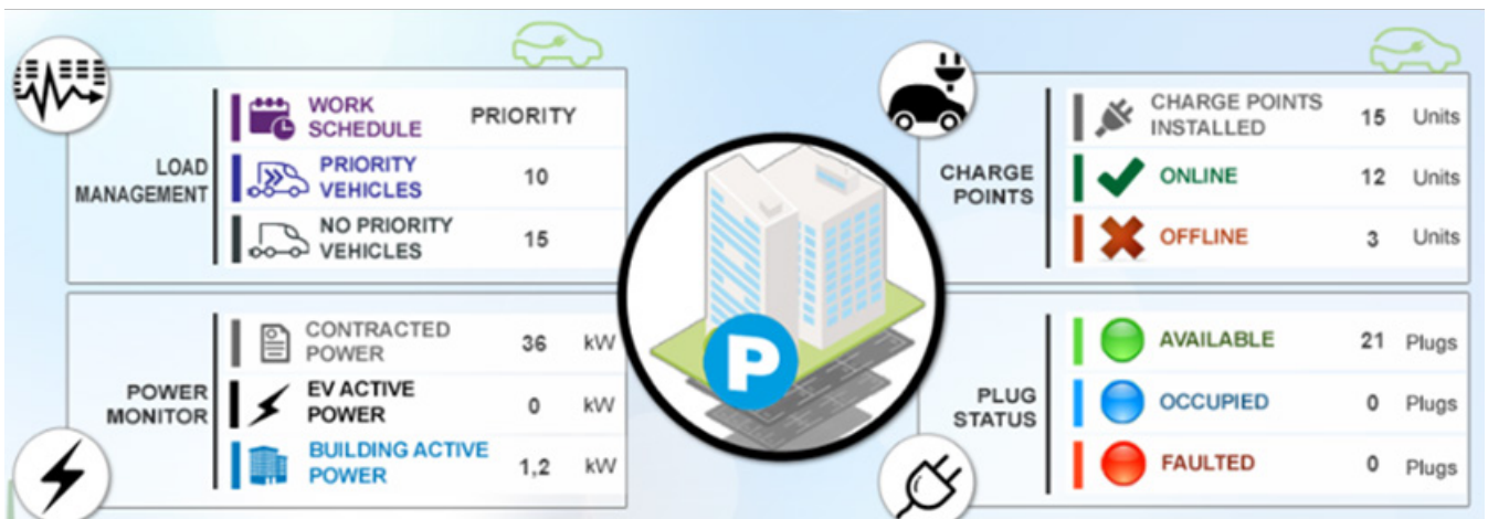
Screen of the main DLM System, where is possible to see the main functions: "Load Management", "Power Monitoring", "Charge Point" and "Plug Status"
